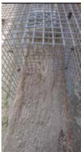
Far-left: The trap is set within a folded 12.5mm (½ inch) wire mesh baffle cradle and screwed to the rail. Note the 51mm x 51mm apertures either side of the treadle plate, which is painted grey and ‘textured’ with soil.
