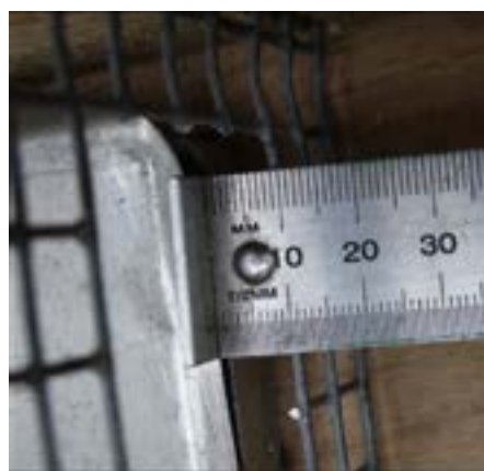
The distance from the edge of the trap plate to the inner baffle(s) must be no more than 10mm, but be careful not to get it so close that the trap doesn't fire properly.
