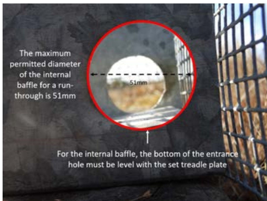
The circle shows legal requirements of the baffle arrangement for a run-through DOC trap. In this case, a DOC 150 trap fixed within a folded sheet metal trap cradle. If you are using wire mesh for the baffle, the square-hole cut-out must be equivalent, ie. no larger than 51mm (2 inch) square. (For a single-entry trap, the hole can be up to 65mm (2½ inch).
