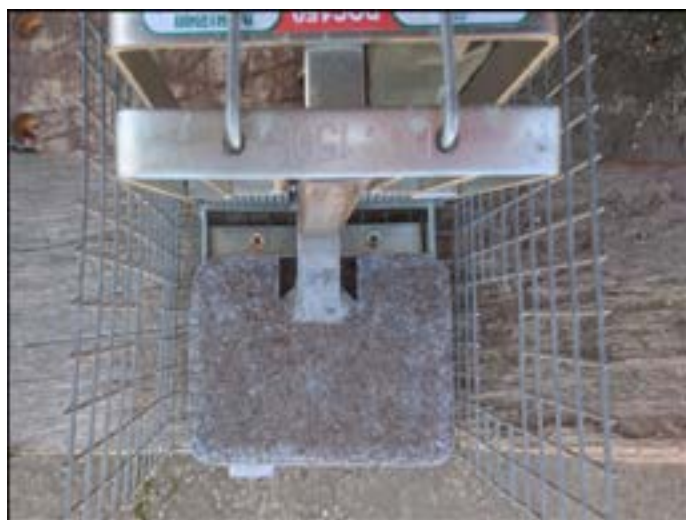
DOC 150 traps lend themselves to being used on rails, but it is imperative that every effort is made to exclude non-targets, as well as ensuring the correct gaps between treadle plate and tunnel side and between trap and inner baffle are maintained at no more than 10mm.
